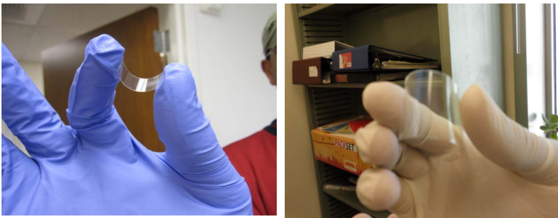
Figure 2. Images of highly transparent and intrinsically defect-free nanoporous morphology as prepared porous alumina membranes.
